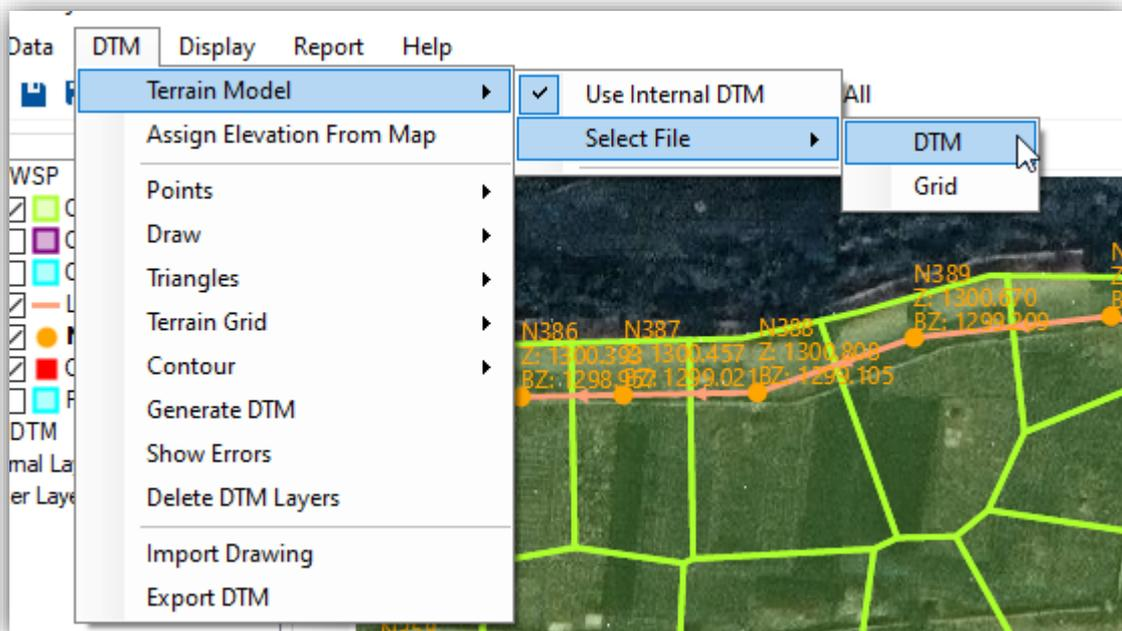
This sub-menu specifies the terrain file to be used for design. The terrain file may be an internal DTM or external DTM/Grid file. If the data is processed and DTM is created within the software, the "Internal Dtm" can be used. Otherwise, external DTM or Grid can be imported for the terrain data.
