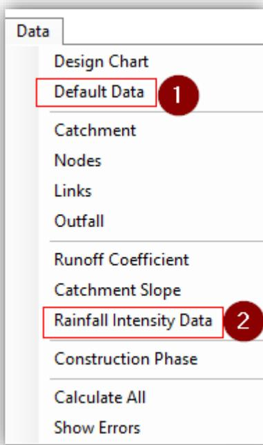
Default Data will be used as criteria for design (minimum cover to pipe, minimum flow velocity, maximum flow velocity, etc.) and values if we do not supply the data (Catchment slope, manning's n for Pipe, etc.)
